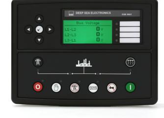
The DSE**8661** is an intelligent controller with automatic transfer switch capabilities that will control breakers up to 1.2 km apart. Using one control module on each breaker, the modules are linked by RS485 and work in unison detecting the incoming supply as well as activity on the line.
